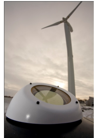
Figure 2c: 2D Steerable scan head on top of short-range WindScanner.
