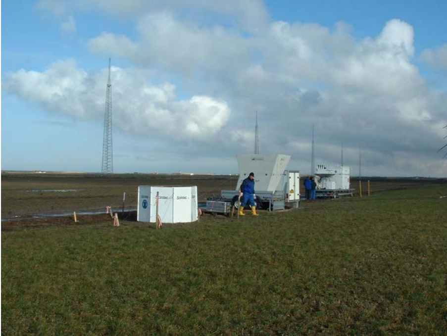
Figure 1 Commercial available SODARs being inter-compared at the Danish Høvsøre test site during the WISE 2004 experiment: An array of SODARS (and one LIDAR) during inter-comparison and testing against the tall met towers (up to 168 meter above ground) equipped with calibrated cup anemometers at several heights. Venue: The Test station for large wind turbines, Høvsøre, Denmark.
