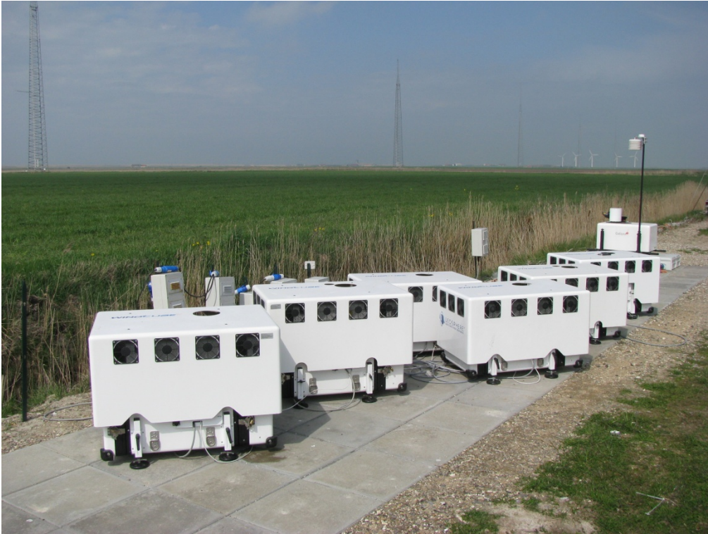
Figure 7: Pulsed wind LIDARs (six WLS7 WindCube's) and one Galion (far back) during testing at Høvsøre
