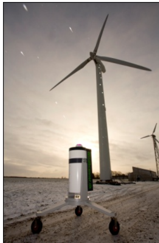
Figure 9b: A Short-Range WindScanner (R2D1) during field test at Risø DTU
