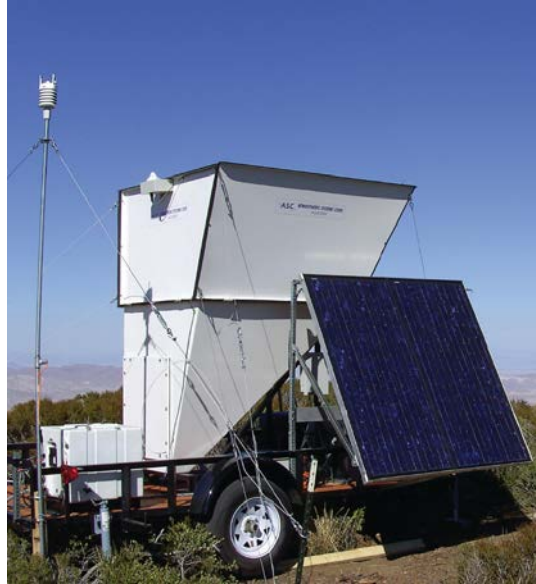
Figure 2. Four of the SODARs designed primarily for wind energy applications. Second Wind Triton SODAR (upper left), AQSystem AQ500 SODAR (upper right), Metek PCS.2000-24/LP (lower left), and ASC 4000i (lower right).
