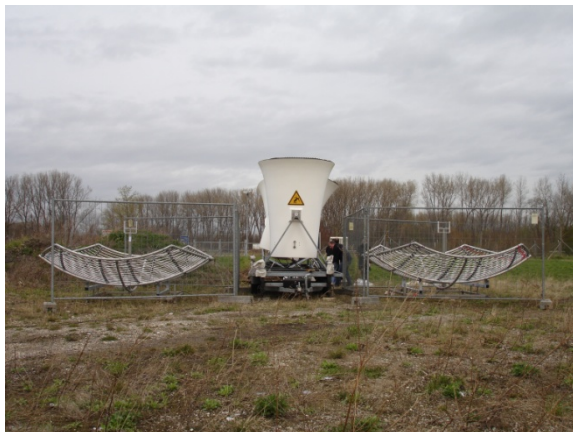
Figure 14.6 Sodar-RASS. The acoustic antenna is in the middle, the electro-magnetic antennas to the left and right.
