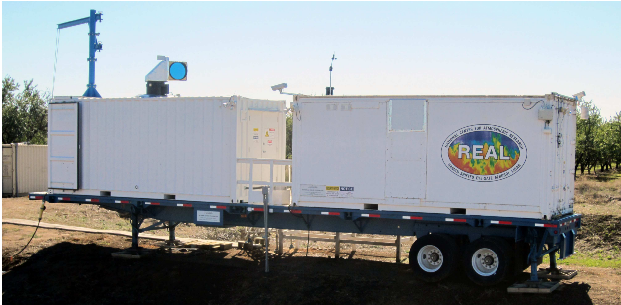
Figure 2: Photo of the NSF/NCAR Raman-shifted Eye-safe Aerosol Lidar (REAL) located at the California State University Chico farm. The lidar resides only in the shipping container on the left. Although all atmospheric lidars must detect backscatter to perform their intended function, the REAL provides the required combination of (1) eye-safety, (2) invisible beam, (3) rapid scanning, (4) continuous operation, (5) high sensitivity to small changes in aerosol properties, and (6) high temporal and spatial resolution data. It does this by transmitting laser pulses with sufficient energy to generate strong SNR backscatter for several kilometers range without any temporal or spatial averaging. In 2012, we expect to complete software that enables the REAL to produce vector flow fields such as those shown in Figs. 19 and 20 in real-time. A discussion of the software to perform the calculation in real-time is given in section 8.5.
