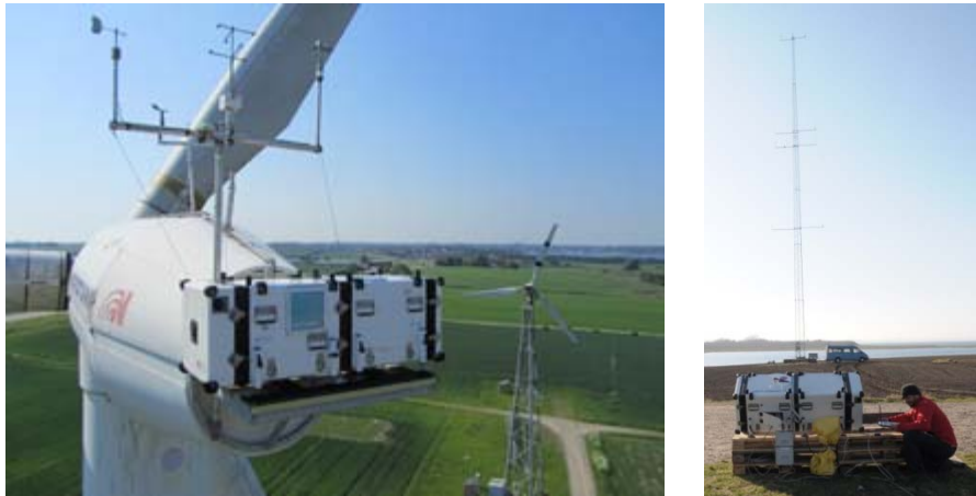
Figure 18, 19. Test site at Risø-DTU with the Nordtank and Tellus wind turbines (left). Tilted SWE Lidar system pointing to a met mast (right)
