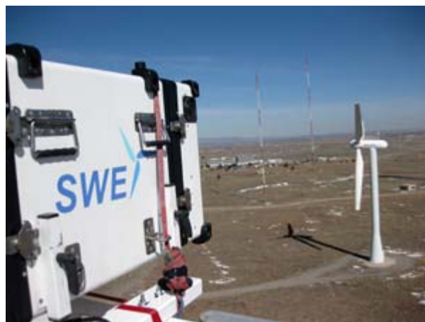
Figure 20. SWE scanner mounted on the CART-2 machine for Lidar Assisted control purposes
