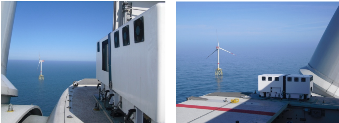
Figure 21, 22. Lidar system (scanner unit and Windcube) on the top of a Repower 5M measuring the inflow
